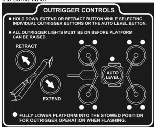
Figure 3-3. Outrigger Controls
